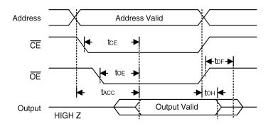
Figure 1. A.C. waveforms for read operation
