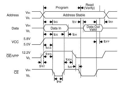
Figure 2. Programming waveforms
