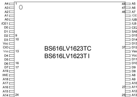
48-pin 12mmx20mm TSOP1 top view
