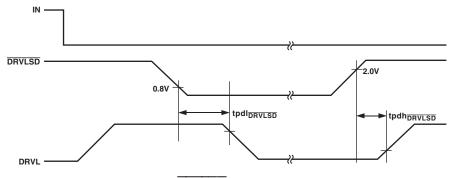
Figure 3. DRVLSD Propagation Delay
