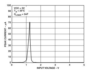
TPC 3. Input Voltage vs. Input Current
