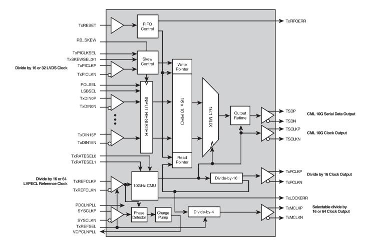
The **BCM8128** is a fully integrated MSA-compliant quad-rate SONET/ SDH/10GE transmitter operating at OC-192 (9.953 Gbps), 10GE (10.3125 Gbps), 10GFC (10.513 Gbps), and FEC (Forward Error Correction) data rates (10.664/10.709, 11.096, or 11.31 Gbps) with serializer and Clock Multiplication Unit (CMU). The low-jitter LVDS interface and onboard low-jitter PLL exceed Optical Internetworking Forum (OIF), IEEE 802.3ae, Telcordia, ANSI, and ITU-T jitter standards.
